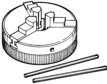
NOTE: The P/N 1042 chuck is threaded 22 x 1.5 mm for use on ER-16 collet spindles.
